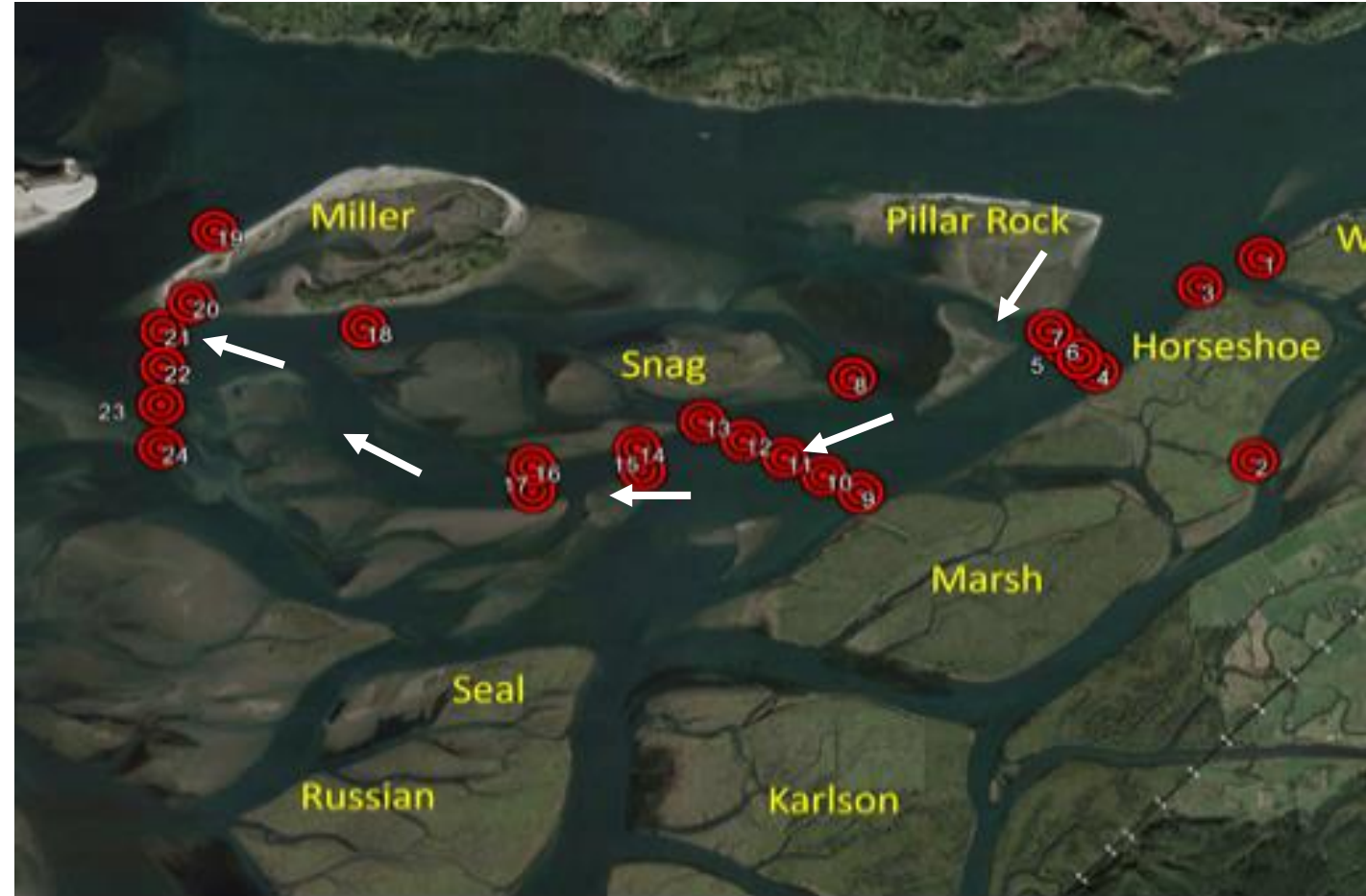
Proposed JSATS autonomous hydrophones arrays near Woody Island Channel.
